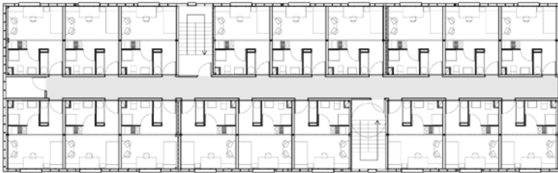
RESIDENCE ETUDIANTE : 18 LOGEMENTS = 12 CONTAINERS
