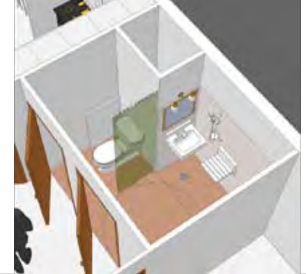
SALLE-DE-BAINS ACCESSIBLE PMR
